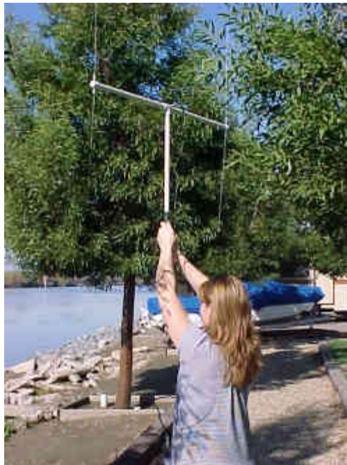
Figure 4.4 - A typical dual-antenna RDF in use.
