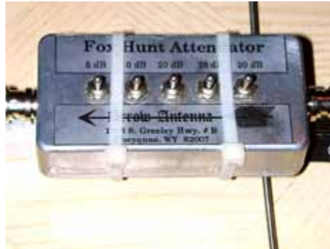
Figure 4.6 - A typical attenuator
