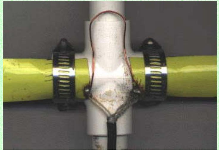
I used 1 1/2 inch hose clamps to attach all the elements on my prototype beam. Others who have duplicated my design have used self tapping screws to attach the elements to the PVC crosses and tees. Performance is the same using either method. The screws are much less expensive but they do not hold the elements as securely. If you do not use 1/2 inch PVC fittings but instead use 3/4 inch, make sure the hose clamps you buy are large enough to fit.
