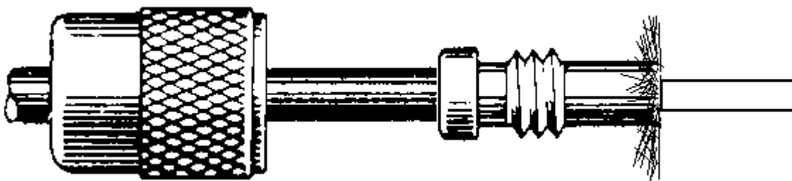
Figure 4 - Coax cable preparation. The 1/4" braid length is approximate and can be longer - it will be trimmed later.
