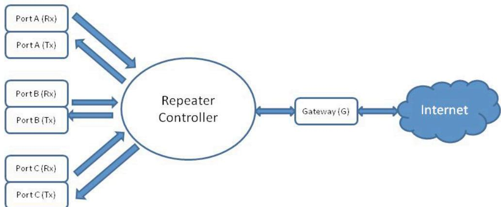
This figure shows 3 RF voice ports (labelled A, B and C - see below) and the gateway connecting the repeater controller (which connects all of the repeater ports together) to the Internet which is used to carry the D-Star network. The figure does not show a data port
