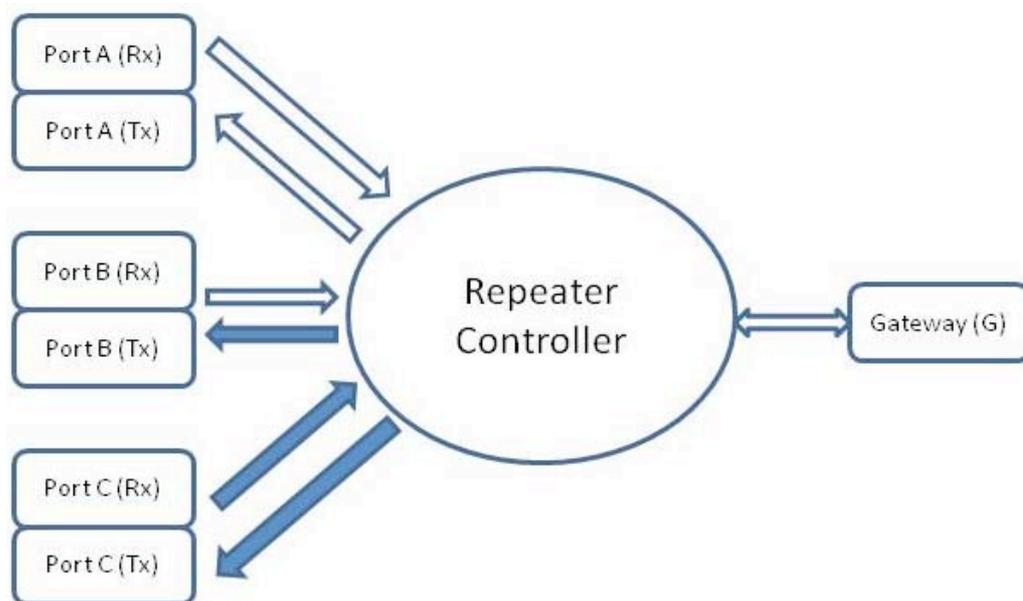
To do this I have to tell the local repeater that I want to send my signal within the repeater from the C port to the B port. I do this by setting the Repeater1 call sign to the C port of the local repeater, and the 'Repeater2' call sign to the call sign of the B port.
