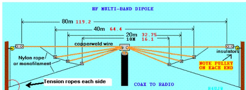
Tension rope is not tied to pulley rope in picture. It is tied near location of pulley rope down on supports within easy reach. It is tied last after final SWR adjustment and the antenna is in it's final position.
