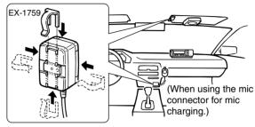
The installation clip can be oriented in 1 of 4 ways.
