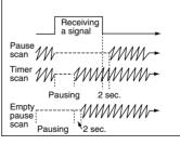
5 resume conditions are available: 3 timer scans, pause scan and empty scan. When receiving a signal, pause scan pauses until the signal disappears; timer scans pause for 5, 10 or 15 sec. Empty pause scan pauses until a signal appears.
