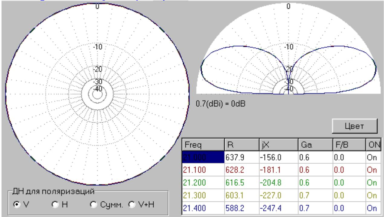
SWR at 15 meters FOR 4B- W3DZZ Antenna
