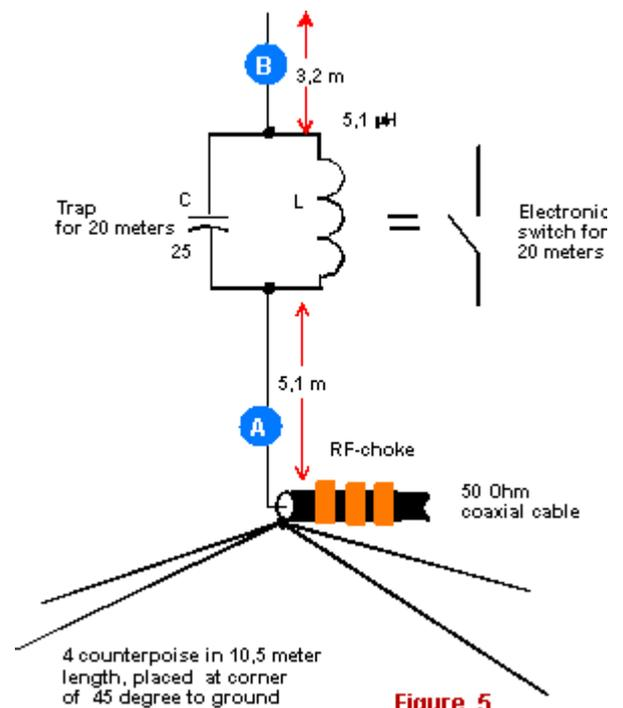
**Figure 5** A four-band trap vertical antenna
