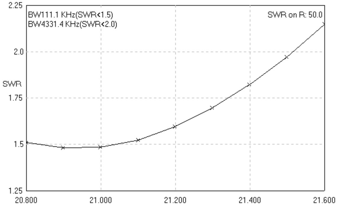
antenna with electrical length in  $\lambda/2$  (having physical length bit less than  $\lambda/2$ ) has input impedance less than 75 Ohms and maybe, close to 60- 50-Ohms, see **Figure 3B**. So, for feeding a dipole trap antenna a 50-Ohms coaxial cable can be used with a high efficiency.
