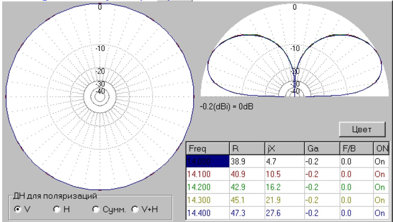
SWR at 20 meters FOR 4B- W3DZZ Antenna
