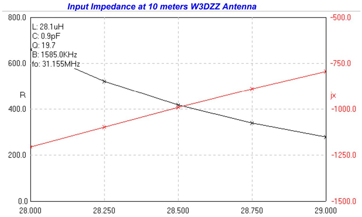
Antenna W3DZZ has input impedance close to 60 Ohms at 80 and 75 at 40, , so, a 75-Ohms coaxial cable can be used for feeding of the antenna.
