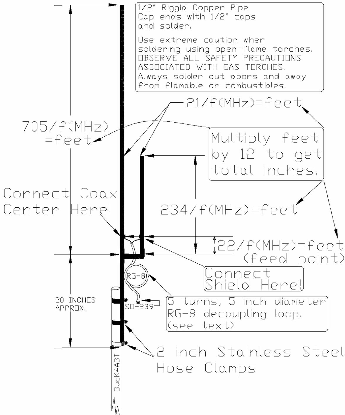
Notice how the decoupling loop is formed from a length of the coax coiled into a 5 turn, 5 inch diameter loop. The coil is then attached it to the mast as shown above. For the final touch, attach an SO-239 (female) coax connector; see text.
