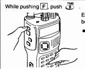
Each push of the key changes the scan resume condition between the two listed beneath.
