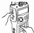
The keys must be pushed within 1.5 seconds of each other to open the DSQ of the other station.
